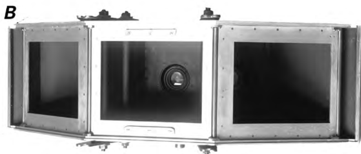
Figure 26. — Cameras developed by James W. Bagley, a USGS topographer, for use in Alaskan topographic surveys. A , Bagley panoramic camera used by USGS topographers in many Alaskan surveys prior to the First World War. 1926 photograph by R.H. Sargent (see USGS, 1929) from USGS Photographic Library, Denver, Colo.; B , Bagley 3-lens T-1 camera used in systematic Alaskan aerial photographic surveys in 1926 and 1929 by the USGS-U.S. Navy Alaska Aerial Survey Expedition. Photograph Moffitt 729 from the USGS Photographic Library, Denver, Colo.
